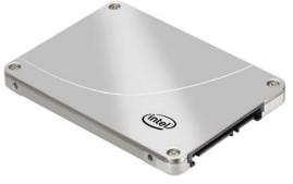
Hard drive speed—the rate at which the storage drive allows you to write data to it and read data from it—affects Solid-Works modeling sessions dramatically, especially when a single drive is used for data storage, Windows operations, and swap. Newer solid-state drives (SSDs) yield better performance than older spindle-equipped hard drives, whose speed is measured in revolutions per minute (hence, RPM).
