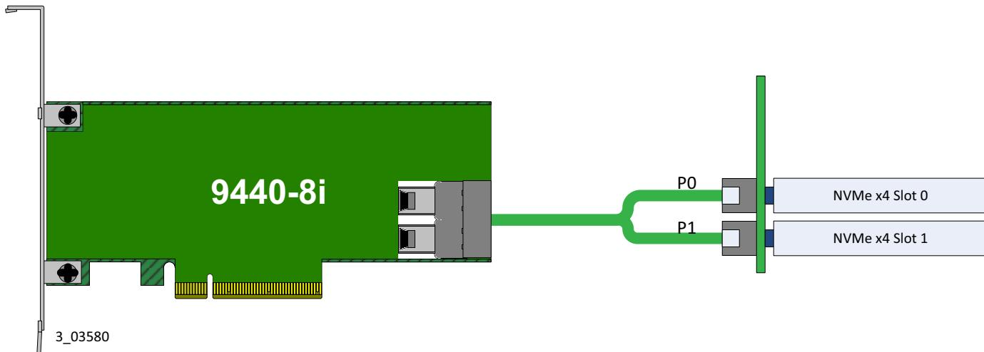
Each leg of the U.2 Enabler Cable needs to connect to adjacent drives; otherwise, the LEDs might not work properly. It does not matter which leg of the cable is plugged into which connector pair as long as adjacent pairs are used. For more information on NVMe LED functionality, please refer to the *Broadcom MegaRAID and HBA Tri-Mode Storage Adapters User Guide*.
